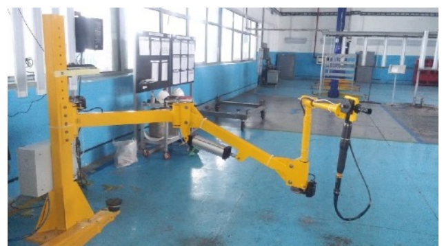
ARM manipulator design: 1- Column, 2- Brake disk No. 1, 3- Brake caliper No. 1, 4- Arrow
