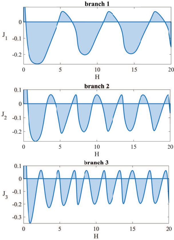
Fig. 6: The stability region (colored) of  $\phi_j$  in the physical plane  $(J, H)$  for type II solutions and the same parameters as in fig. 3.
