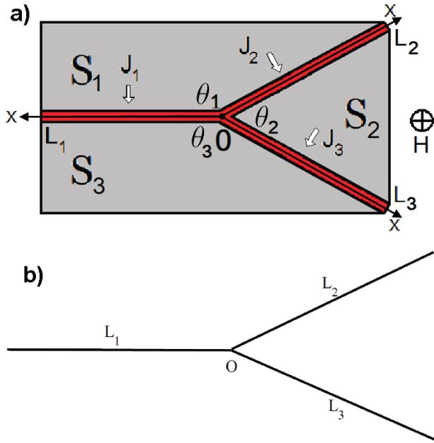
Fig. 1: (a) Branched Josephson Y-junction in a constant magnetic field,  $H$ . Red lines imply normal metal or insulator.  $J_1, J_2$  and  $J_3$  are the Josephson currents flowing through each branch of the junction. (b) Basic star graph.  $L_j$  is the length of the  $j$ -th branch of the graph ( $j = 1, 2, 3$ ).
