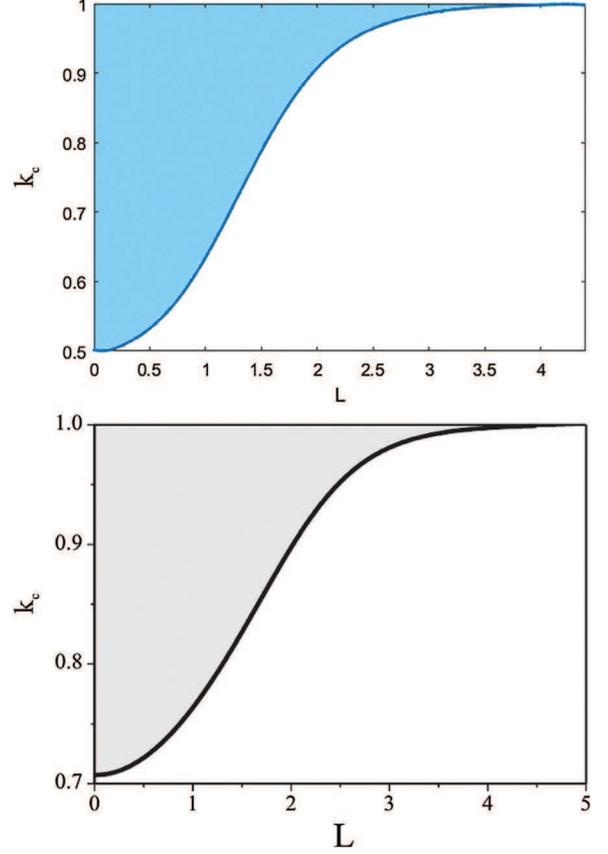
Fig. 2: Upper panel: The dependence of the stability border,  $k_c = k_c(L)$  on the branch length (solid line) for the branched Josephson junction. The colored area corresponds to the stability area. Lower panel: similar plot in the linear (unbranched) case from ref. [21].
